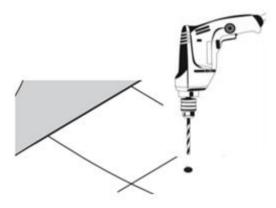
7. If fitting into a solid floor, you will need to install the screw plugs and tap flush to the floor, then place the brackets over the drilled holes/plugs and insert the screws and washers through the brackets and secure into position.
