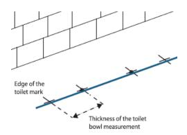
5. If using the 'L' shaped bracket assembly, place the front edge of the bracket on the inside mark, then mark the screw hole position to secure the bracket to the floor. Repeat on the other side.
